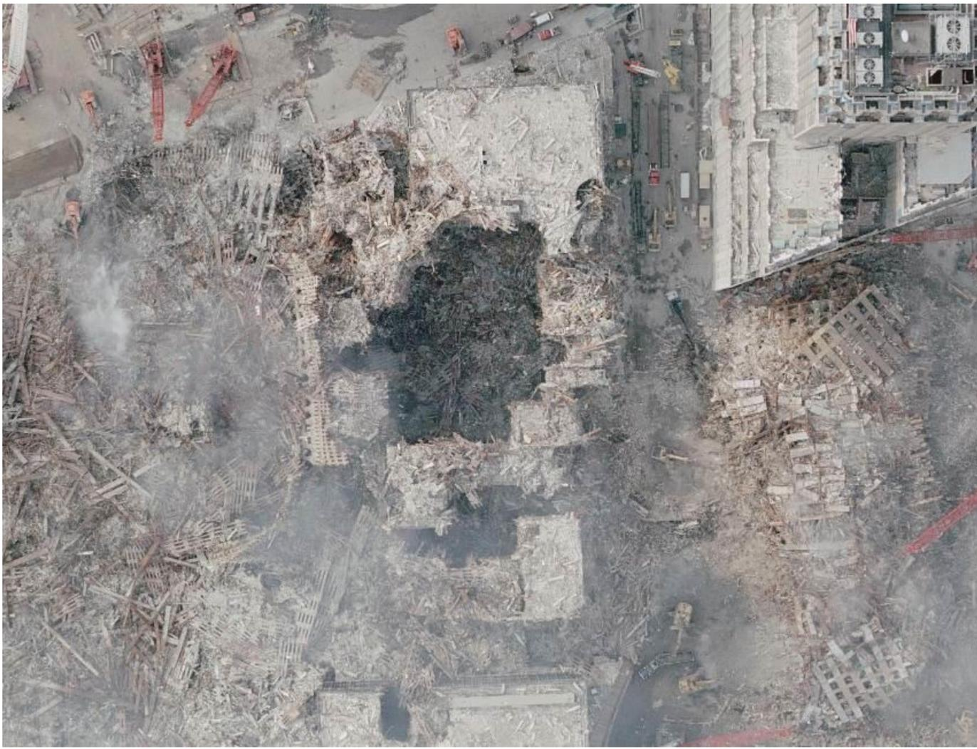
70 Various water sources were present at the WTC site after September 11 (rainfall, water used for firefighting, water that leaked via two WTC cooling water lines from the Hudson, and water that leaked from main water lines). Most water drained into the Port Authority Trans-Hudson (PATH) commuter line tunnel. The amount of water that was drained from the WTC site has been estimated based on pumping records. See Semkow et al., pages 9 and 10.
