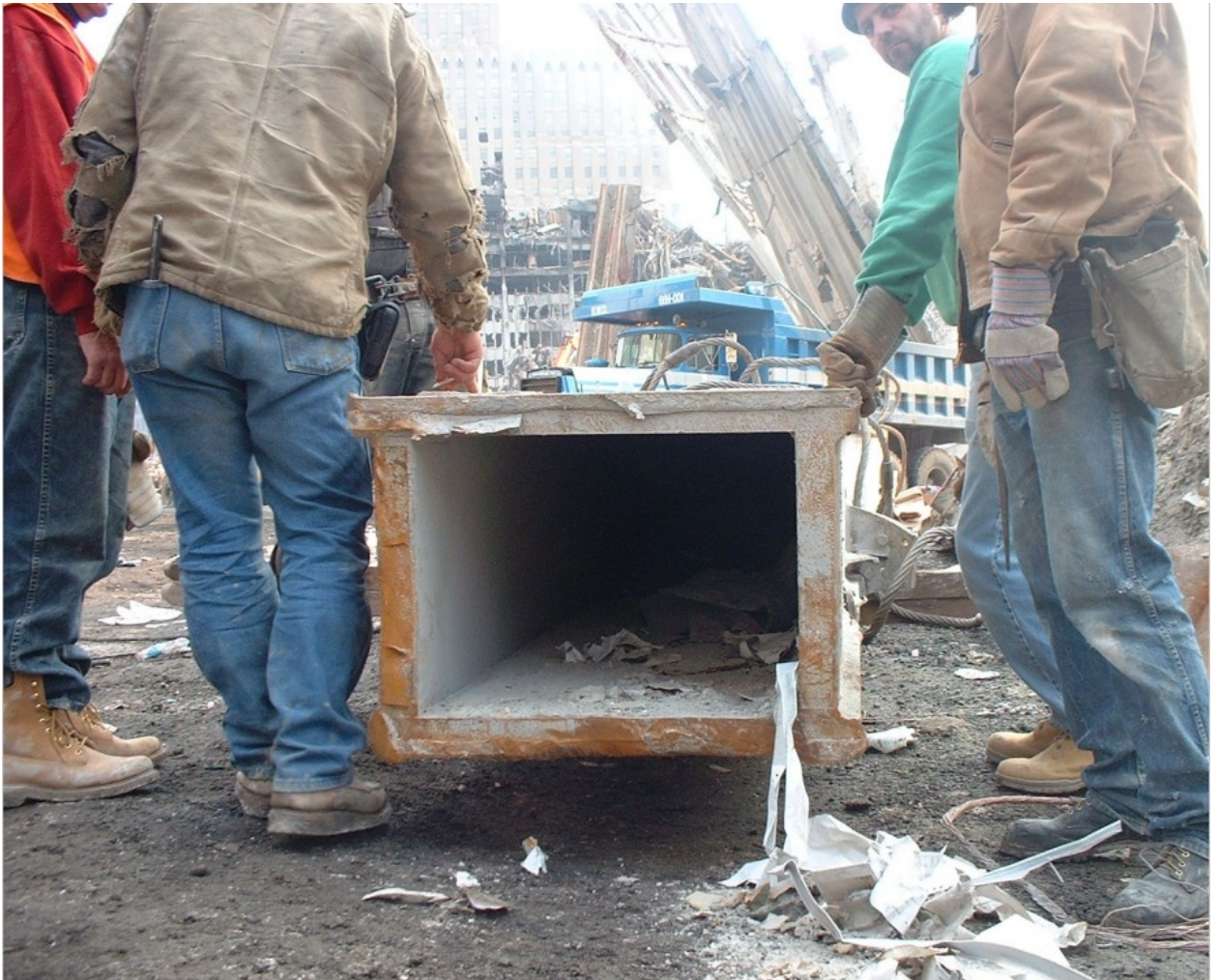
Above – a typical WTC perimeter column at “ground zero”.
