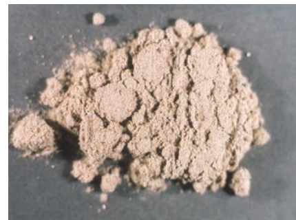
Figure 2. The general appearance of the bulk dust collected at the Market Street location east of the WTC site. Dust samples from the other two sites were similar in appearance. Magnification = 4 \times .
