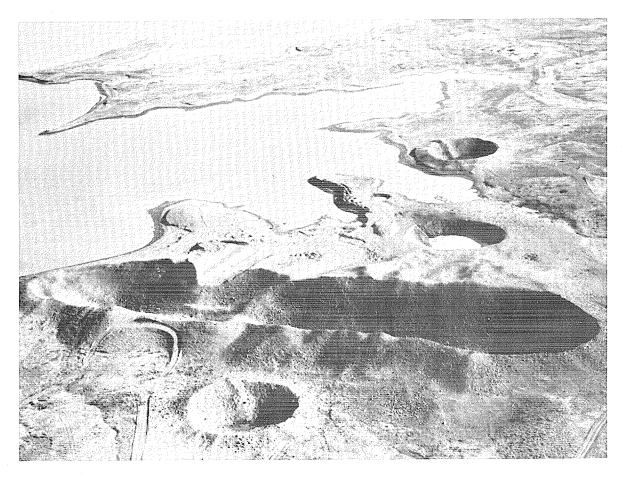
Figure 1. Pre-GONDOLA 20-ton single-charge craters and connecting row crater prior to execution of the reservoir connection experiment.
